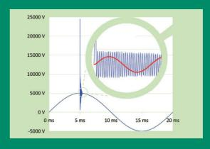
Voltage shape with surge at an MV transformer
