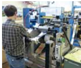
Reactors with cost-saving aluminum coils are produced in band-winding technology.
