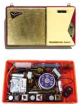
"Sternchen", the first East German transistor radio. The three Elkos from Gera are clearly visible. In the year 1959 alone, 200,000 miniature elkos were put into these devices.
