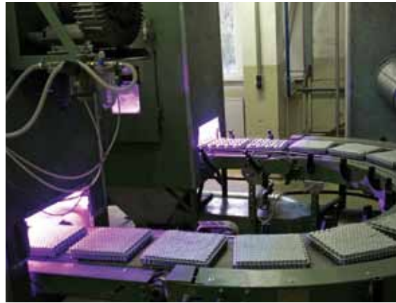
This contact-spray-line from the eighties provided loyal services till 2004. It was efficient for the so-called "mass production" because it could process large quantities of windings in a short time.
