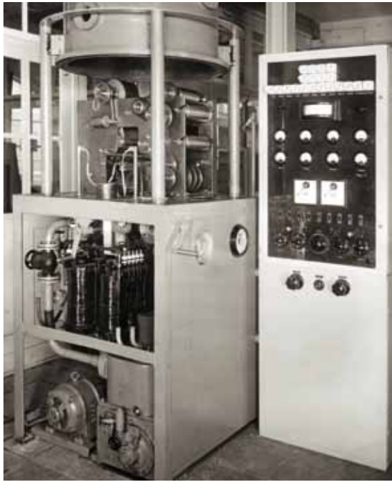
Vacuum chamber for oil impregnation of paper capacitors
