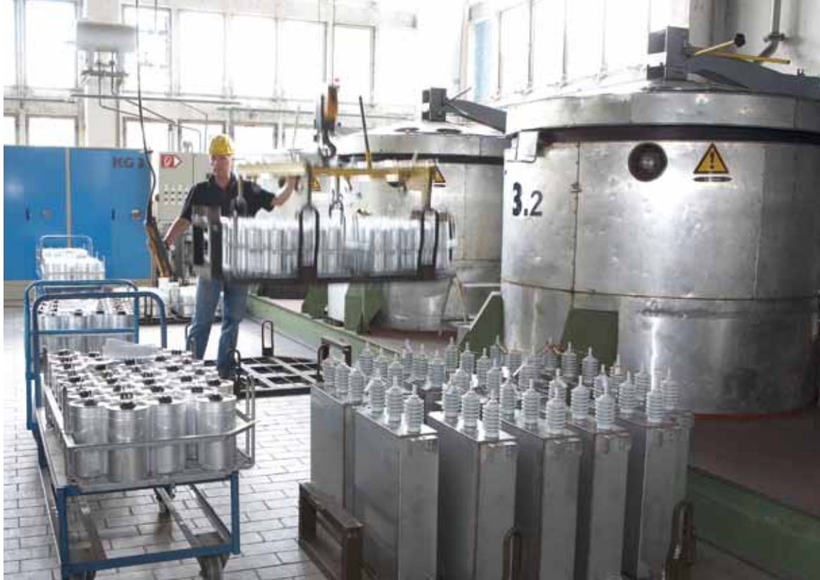
Old chambers with new function: The impregnation chambers from the seventies were given a general overhaul, fitted with new controls and refashioned to serve for vacuum drying.
