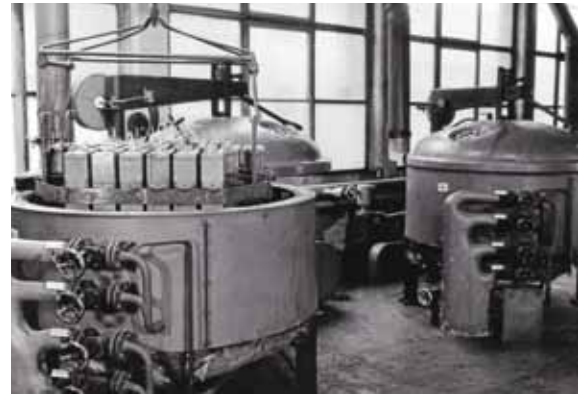
Vacuum chamber for oil impregnation of paper capacitors
