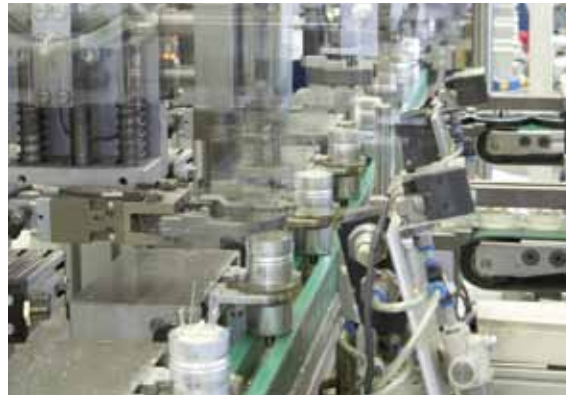
In one go, the Somatic line completes the entire assembly of metal can capacitors including the integrated pressurefuse.
