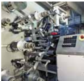
Only the best for the winding department: automatic winding machine by MAG Hamburg for larger diameters.
