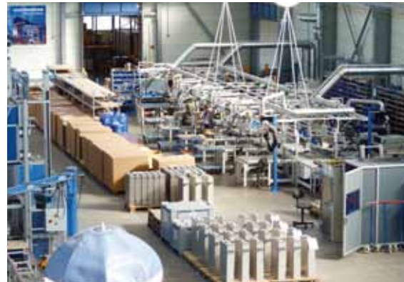
Full house. One single HVDC project often consumes thousands of large capacitors, each weighing about 100 kgs and more.
